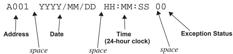
The instrument **Exception Status** codes that the instrument returns for the ASCII protocol are the same as those described for the Modbus RTU protocol in **Instrument Exception Status** on page 75.
