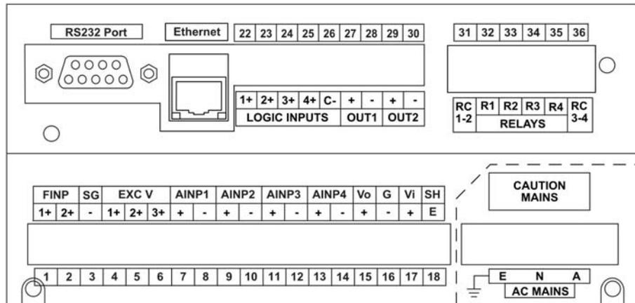
Figure 5 Rear Panel Connections - New Ethernet Version
