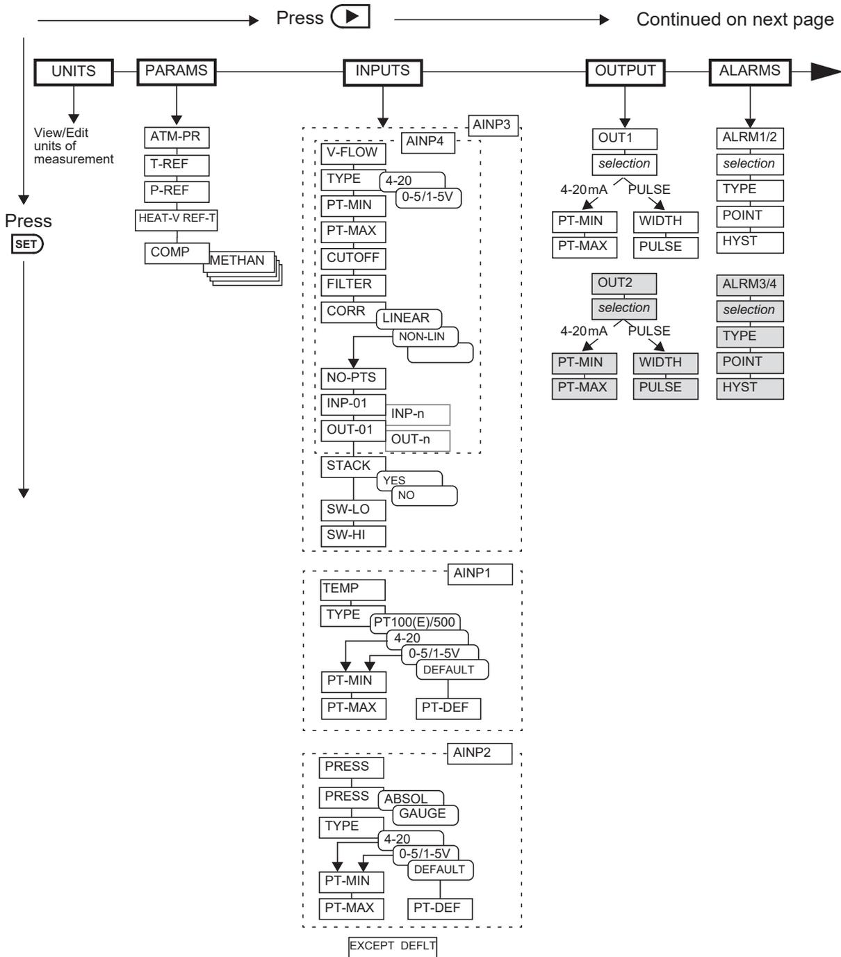
Figure 17 Calibration Menu Tree Sheet 1
