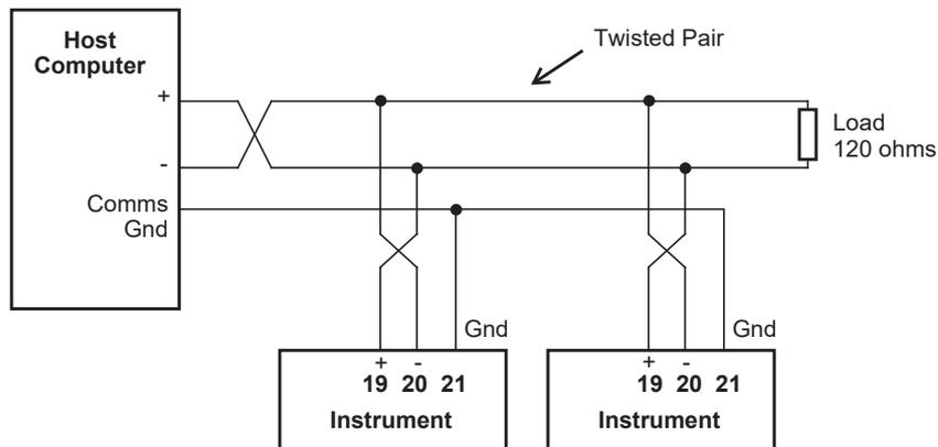
Figure 15 RS-485 Interface Connections
