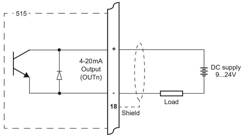
Figure 12 Output 4-20mA Connection Diagram
