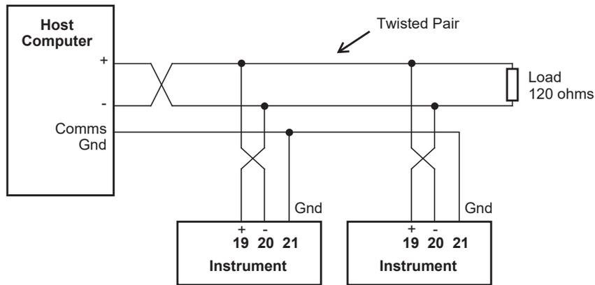
Figure 20 RS-485 Connections
