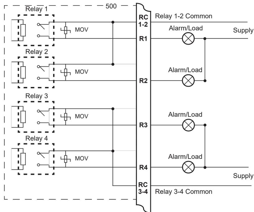
Figure 14 Relay Connection Diagram
