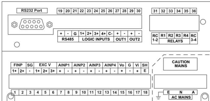
Figure 4 Rear Panel Connections - New RS485 Version
