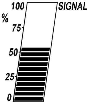
The signal bar graph displays the input signal as a percentage.
