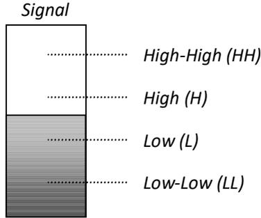
The alarms can be assigned to **signal** or **process variable** which is done during programming (see Section 4.1). Each alarm is individually programmed as a percentage (0-100%) of signal or process variable.
