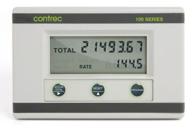
The 102D Rate Totaliser is designed to operate with virtually any pulse/frequency generating flowmeters including Turbine, Positive Displacement, Electromagnetic and Coriolis. The unit is powered entirely from the internal replaceable batteries.
