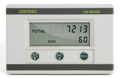
The 102A Rate Totaliser is designed to operate with any flowmeter which produces a 4-20mA output, including Differential Pressure Devices, Magnetic or Vortex Flowmeters. The unit is powered entirely from the 4-20mA current loop.
