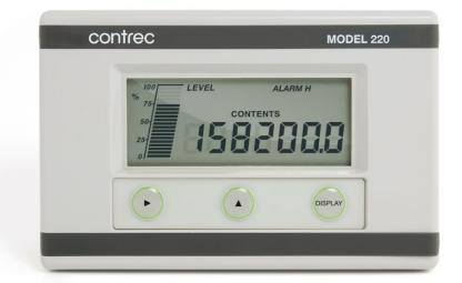
The Model 220 Level Monitor accepts a 4-20mA signal from a wide range of level sensors, including pressure transmitters, ultrasonic sensors or capacitance probes, and displays both level and tank contents on a large LCD display.
