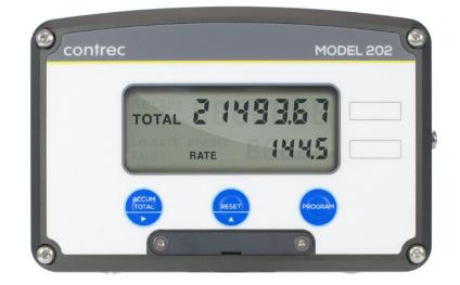
The 202D Field Mounting Rate Totaliser requires no external power and is designed to operate with turbine, positive displacement and paddlewheel flowmeters in applications such as irrigation systems and pipeline measurement, and as a replacement for mechanical registers.
