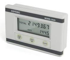
The instrument provides a 2-wire re-transmission of the flow rate. Both the 4mA and 20mA points are fully programmable so that the output can span across the entire range or, alternatively, across a small section of the operating range.
