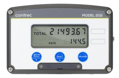
The 202D Field Mounting Rate Totaliser requires no external power and is designed to operate with turbine, positive displacement and paddlewheel flowmeters in applications such as irrigation systems and pipeline measurement, and as a replacement for mechanical registers.
